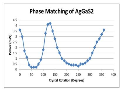
We were able to optimize the power of DFG with the signal at 1450 nm and the idler at 1705 nm. At these wavelengths, the energy split was 66% signal and 34% idler. The wavelength of the DFG beam was 9700 nm and the AgGaS2 crystal was rotated to 134 degrees. As a result of all this, we achieved a maximum power of 10.5 mW.
