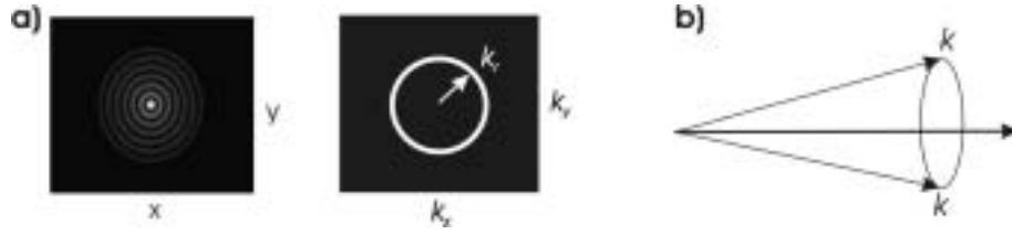
Figure 2. Angular spectrum of a Bessel beam: (a) intensity profile of Bessel beam. With its accompanying angular spectrum – the Fourier transform of the Bessel function is a ring in k -space; (b) shows how the k -vectors of the Bessel beam propagate on a cone.
