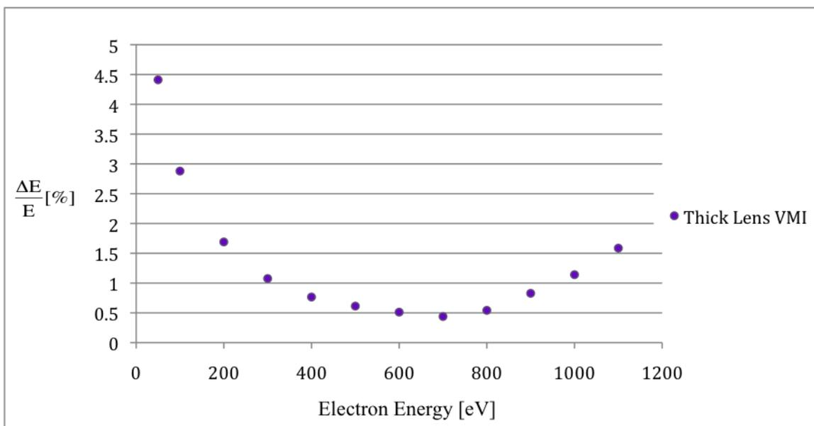
**Fig. [4]:** Resolution versus electron energy chart. The energies for these electrons vary from 50-1100 eV. The voltage magnitude of the repeller electrode is 30 kV. For optimal resolution,  $V_{\text{focus}}$  is set to 2800kV (80% of the repeller voltage).
