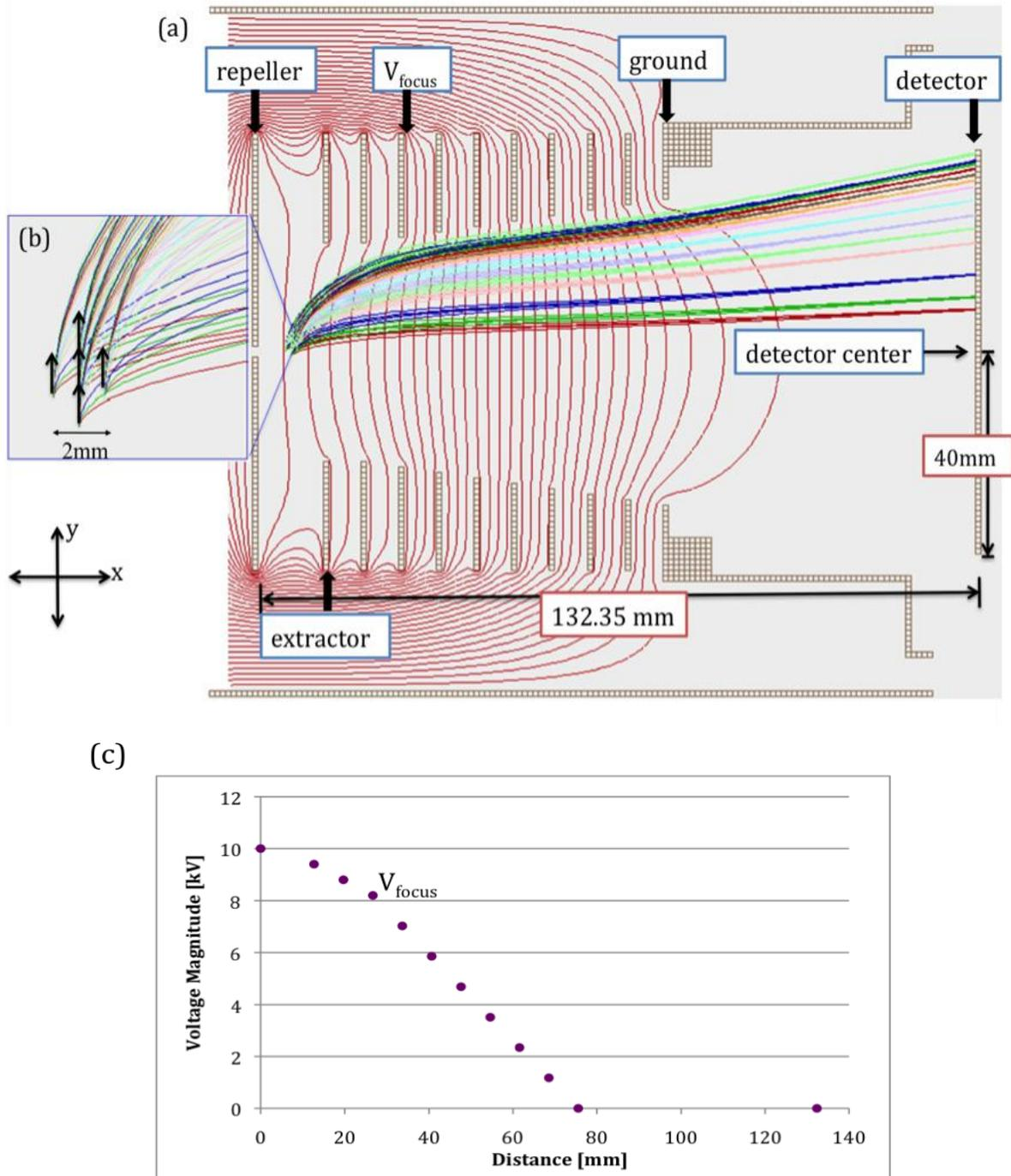
**Fig. [2]:** (a) Diagram of the thick lens VMI. The repeller electrode is set to -10kV and  $V_{\text{focus}}$  is at 82% of the repeller (-8200kV). Electron energies range from 15eV to 360eV. (b) Electrons are projected in the same direction. Diameter of electron spot is 2mm. (c) Distance versus the voltage magnitude of the repeller, extractor,  $V_{\text{focus}}$ , ground, and detector, respectively.
