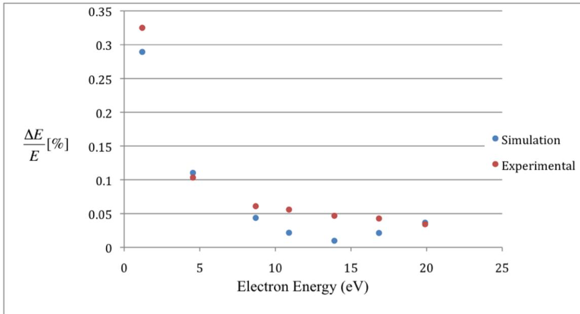
**Fig. [9]:** Resolution versus electron energy for our thick lens VMI simulations and experimental results. The voltage on the repeller was set to -799 V and the electron energies range from 1.2 eV to 19.9 eV.
