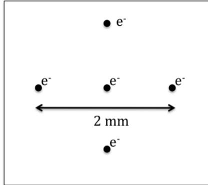
**Fig. [1]:** Initial electron spot size used in our Simion simulations.
