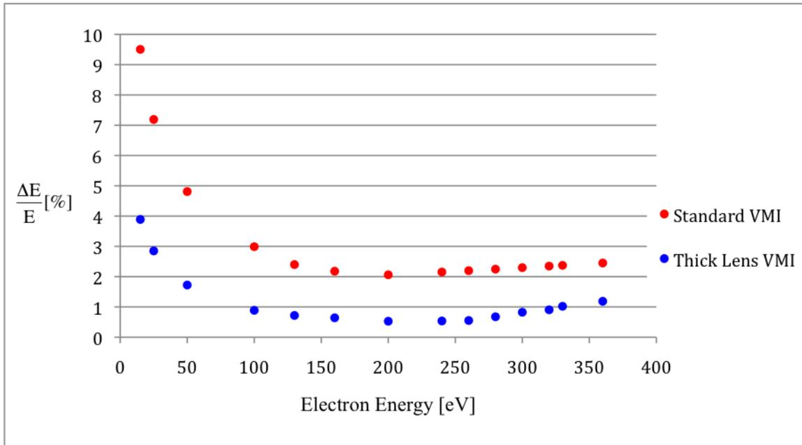
**Fig. [3]:** Resolution versus electron energy chart. The energies for these electrons vary from 15-360 eV. The voltage magnitudes of the repeller electrodes are 10 kV. For optimal resolution in each model, the extractor electrode of the standard VMI set to 9500kV and  $V_{\text{focus}}$  of the thick lens VMI set to 8200kV.
