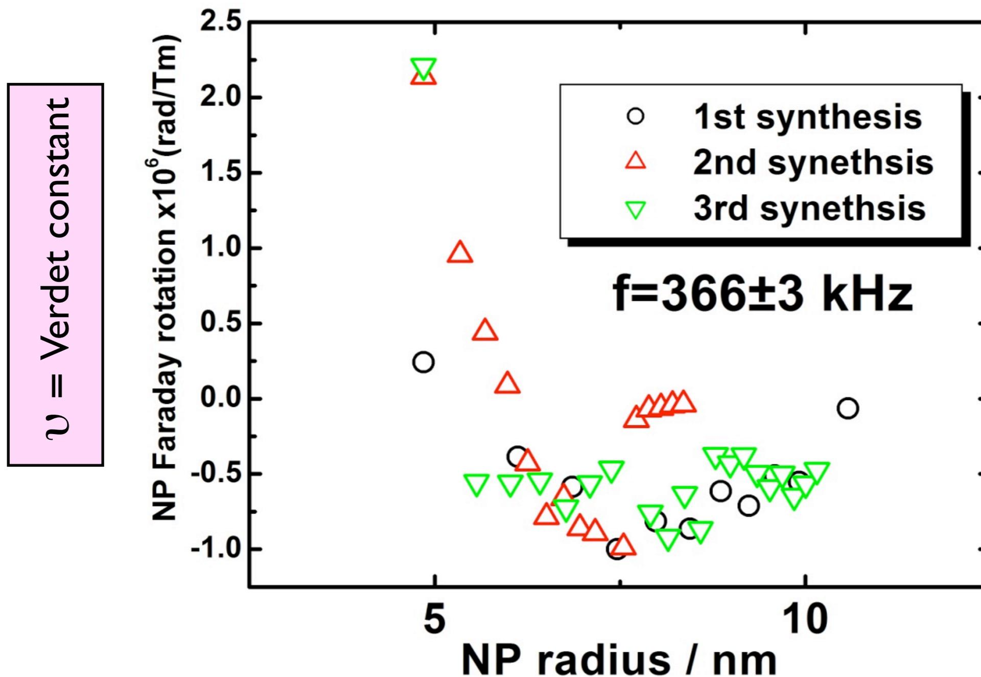
Figure 4 (b) Experimental Verdet constant of gold coated  $\text{Fe}_2\text{O}_3$  nanoparticles only (normalized by the volume fraction of the particles) as a function of gold shell thickness
