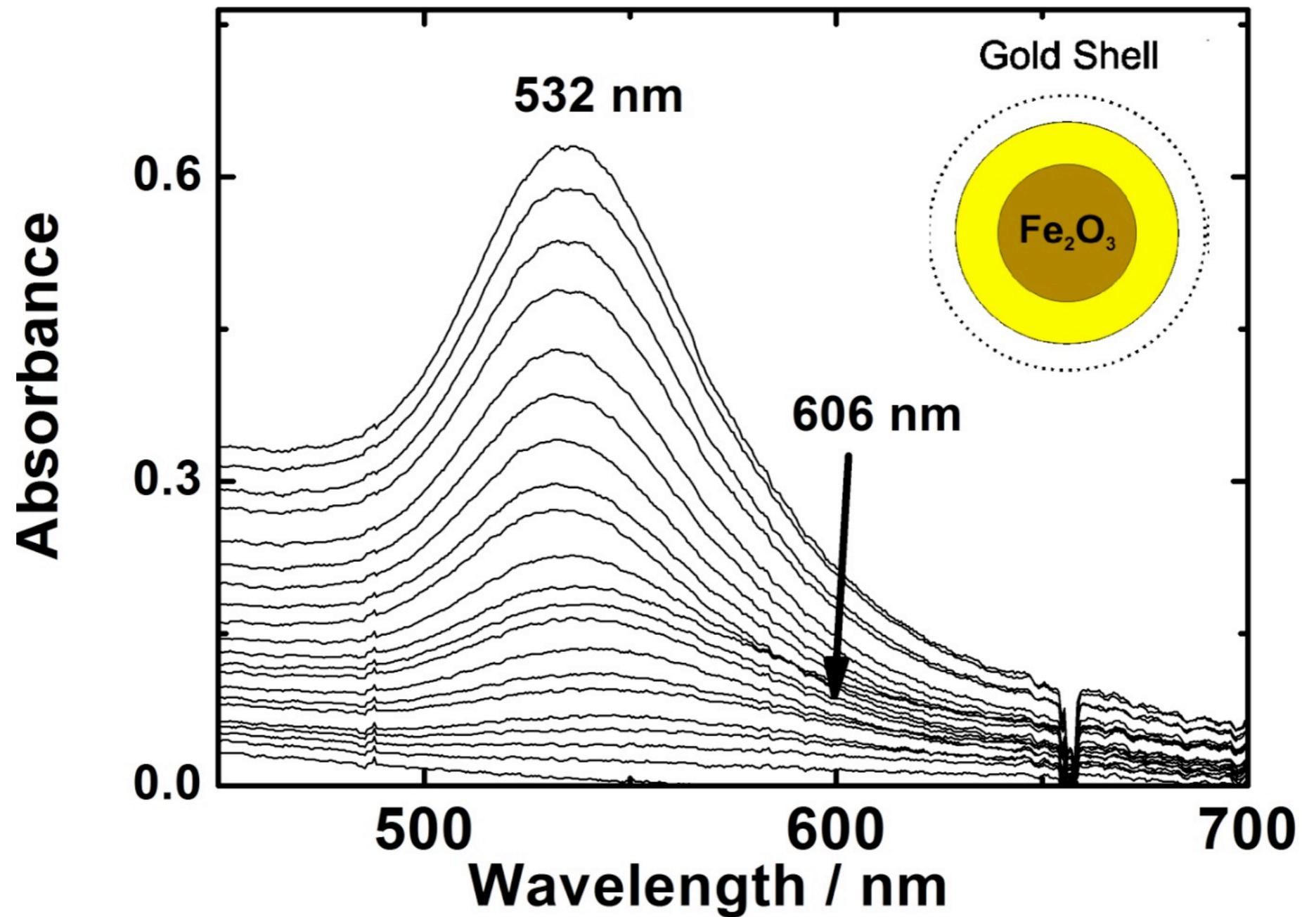
Figure 3 (a) UV-vis absorption spectrum of 3<sup>rd</sup> batch synthesis of gold coated  $\text{Fe}_2\text{O}_3$  nanoparticles. The initial peak position is indicated by an arrow at 606 nm and shifts to 532 nm with increasing thickness of gold shell.
