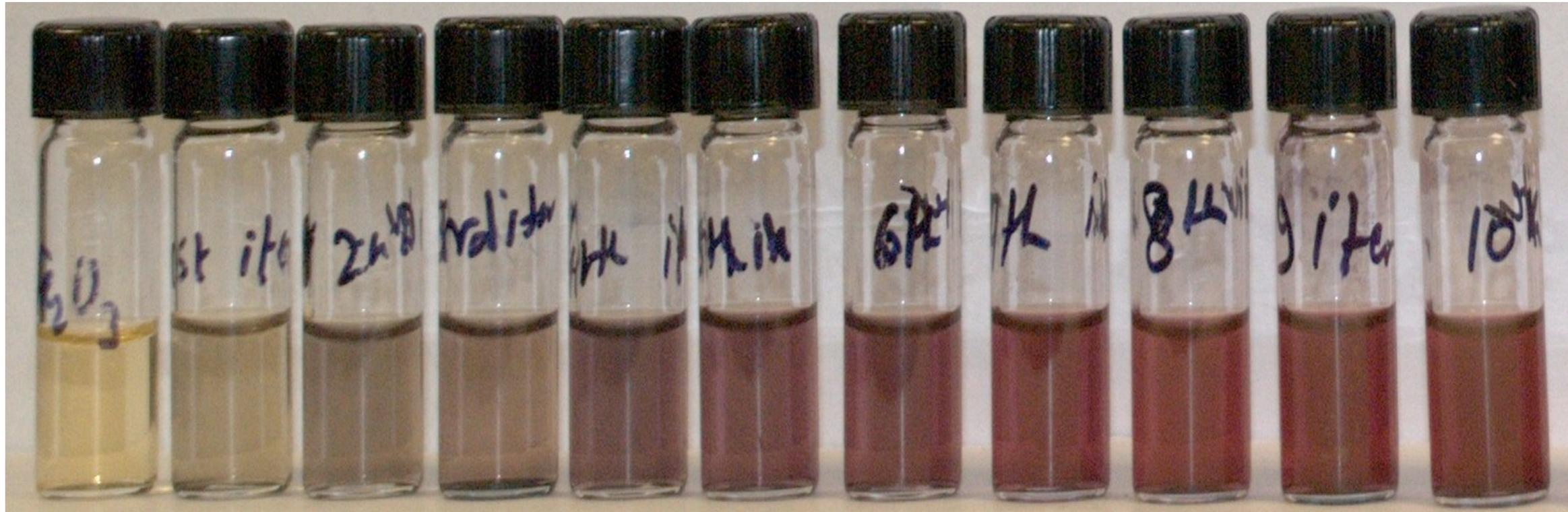
Figure 3 (b) Variation of color change when the thickness of gold onto the surface of the nanoparticles is increased.
