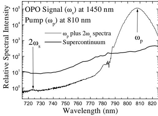
Fig. 2. The input spectrum coupled into the microstructure fiber along with the supercontinuum generated. Although the magnitude of  $2\omega_s$  is five orders of magnitude smaller than of  $\omega_p$ , the mixing of the supercontinuum and  $2\omega_s$  generates a strong beat frequency. The  $2\omega_s$  feature in the above spectrum disappears when the OPO stops oscillating.
