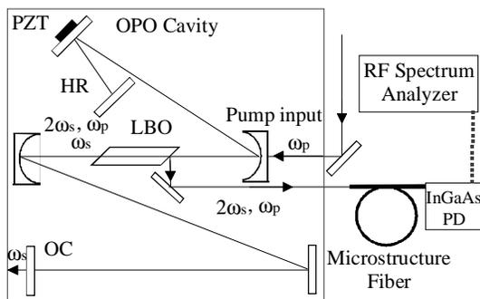
Fig. 1. The OPO cavity showing the pump and  $2\omega_s$  subharmonic reflected from the LBO crystal. Both  $2\omega_s$  and  $\omega_p$  are coupled into the microstructure fiber. The supercontinuum generated by  $\omega_p$  mixes with  $2\omega_s$ , which causes frequency beating measured in the combined signal RF spectrum. HR: High reflector; OC: Output coupler; PZT: Piezoelectric transducer.
