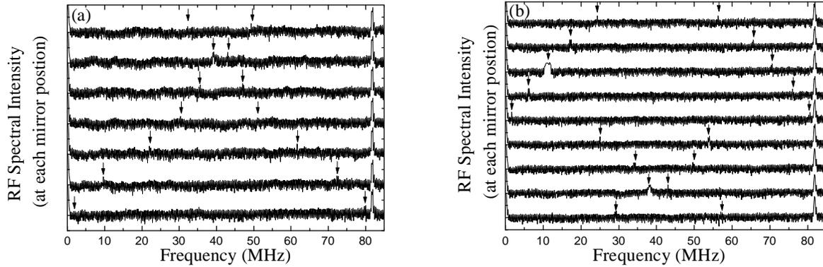
Fig. 3. Control of the beat frequency for OPO signal operation at (a) 1440 nm and (b) 1450 nm. The arrows indicate the location of the beat frequency  $f$  and the sideband  $f-F$  where  $F$  is the repetition rate of the laser ( $F=82$  MHz). Each of the successive RF spectra was taken as the mirror position was changed by  $0.1 \mu\text{m}$ .
