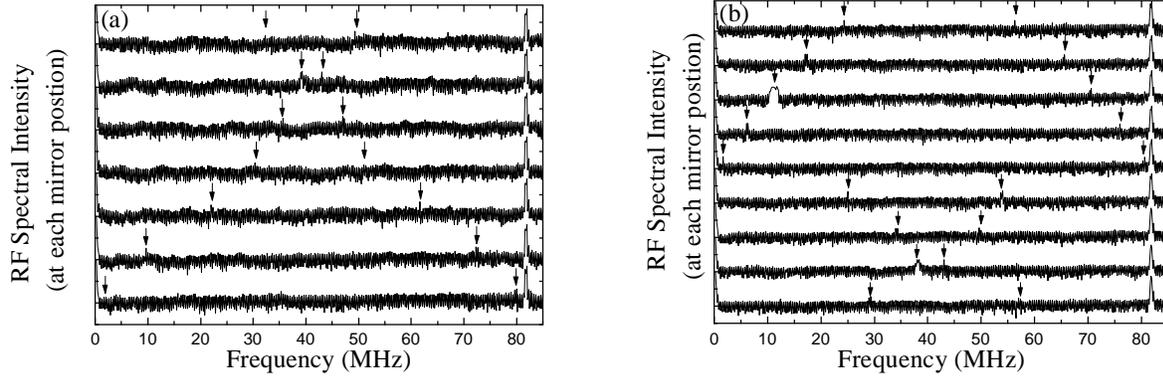
Fig. 3. Control of the beat frequency for OPO signal operation at (a) 1440 nm and (b) 1450 nm. The arrows indicate the location of the beat frequency  $f$  and the sideband  $f-F$  where  $F$  is the repetition rate of the laser ( $F=82$  MHz). Each of the successive RF spectra was taken as the mirror position was changed by  $0.1 \mu\text{m}$ .
