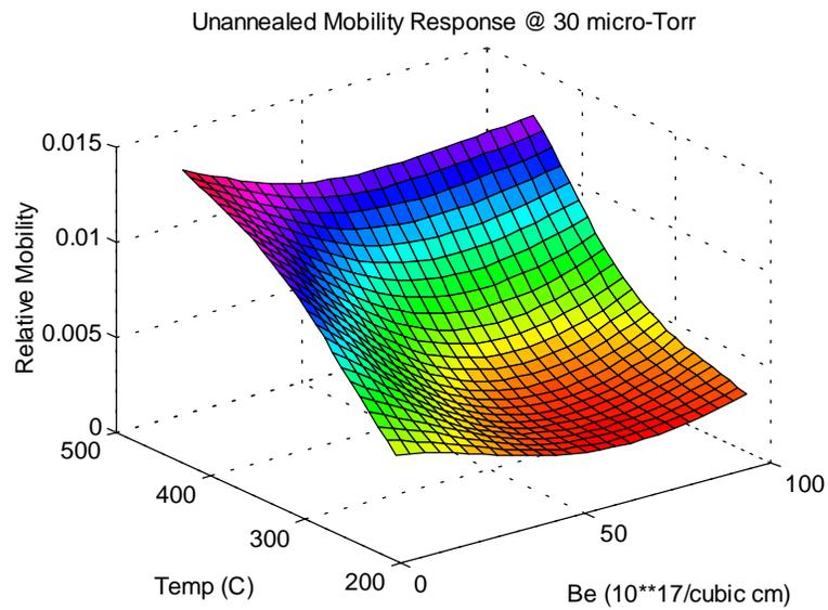
Figure 3. 3D contour of mobility as a function of growth temperature and Be doping for as-grown material at a constant As overpressure of 30  $\mu$ Torr. The contour was generated by a neural process model from data taken via time-resolved terahertz spectroscopy. The growth temperature strongly influences the mobility.
