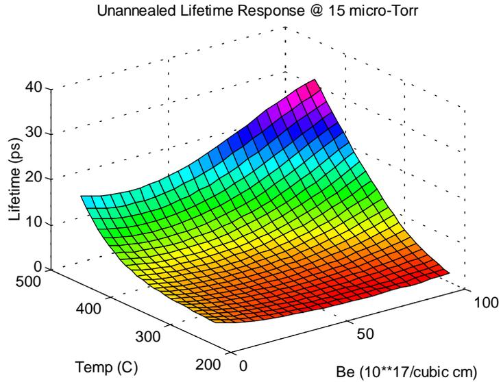
Figure 2. 3D contour of carrier lifetime as a function of growth temperature and Be doping. The contour is for as-grown material grown at 15  $\mu$ Torr As overpressure. The contour was generated by a neural process model from data taken via time-resolved terahertz spectroscopy. Notice that carrier lifetime increases as the Be doping of the material increases.
