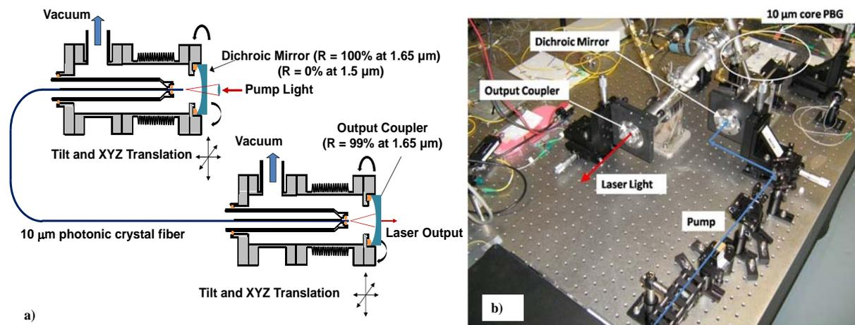
Fig. 1 a) The cavity for the scenario of pumping at 1532 nm and lasing at 1650 nm. b) Picture of the actual cavity.
