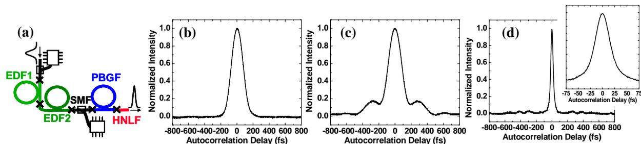
Fig. 1 (a) Parabolic amplifier. (b) Autocorrelation measurement of compressed pulse after the new PBGF that exhibits low dispersion slope. (c) Compressed pulse after Crystal Fibre HC-1550-02 PBGF. (d) Compressed pulse after OFS HNLF.
