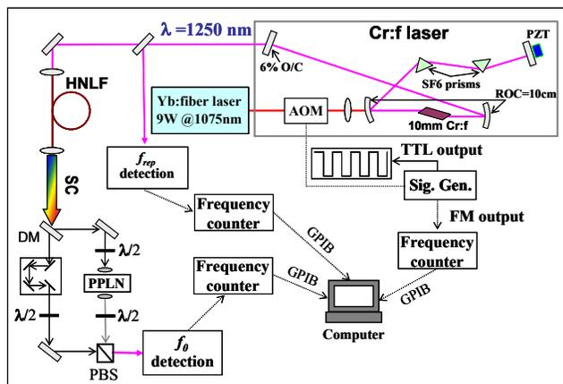
Fig. 1: Experimental configuration used to make  $\Delta f_0/\Delta P$  measurements as a function of relative prism insertion. (DM=dichroic mirror,  $\lambda/2$ =half-wave plate, PBS= polarizing beam splitter, O/C=output coupler, ROC=radius of curvature, Sig. Gen.=signal generator, all other abbreviations are given in the main text)
