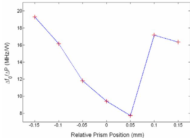
Fig. 2: Preliminary results showing a dependence of the  $\Delta f_0/\Delta P$  signal with the relative prism insertion. A minimum in the  $\Delta f_0$  response of is visible corresponding to a maximum required  $\Delta P$  needed to maintain a fixed  $\Delta f_0$ .
