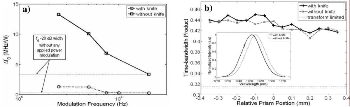
**Fig.2: a)** frequency response of  $f_0$  width to fast power modulation with (dotted) and without (solid) the knife edge. **b)** Time-bandwidth product for our Cr:f laser with (thick dotted) and without (thick solid) the knife edge inserted compared to the transform limited case (narrow dotted), inset shows the difference in the power spectra with (solid) and without (dotted) the knife edge inserted.
