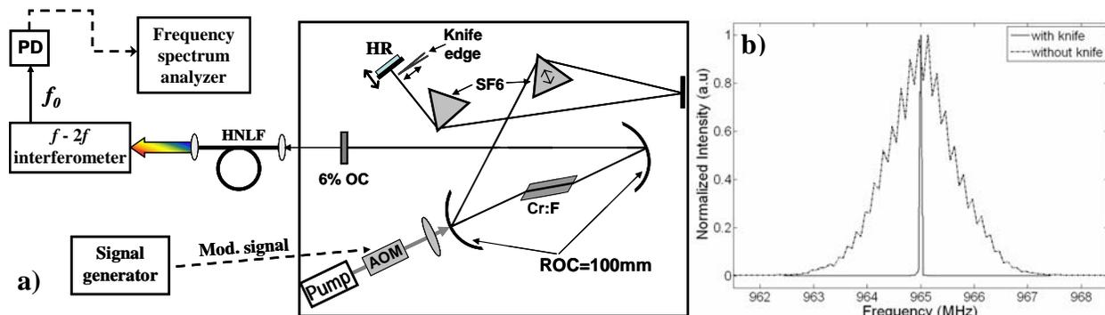
**Fig.1: a)** Cr:f laser cavity and  $f_0$  detection configuration showing the knife edge, with HR = high reflecting endmirror, OC = output coupler, PD = photodetector. **b)**  $f_0$  linewidth plots with the knife edge inserted (solid) and without the knife (dotted).
