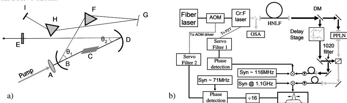
Fig. 1. a) Laser cavity configuration. b) Servo control schematic used to lock  $f_r$  and  $f_0$ .
