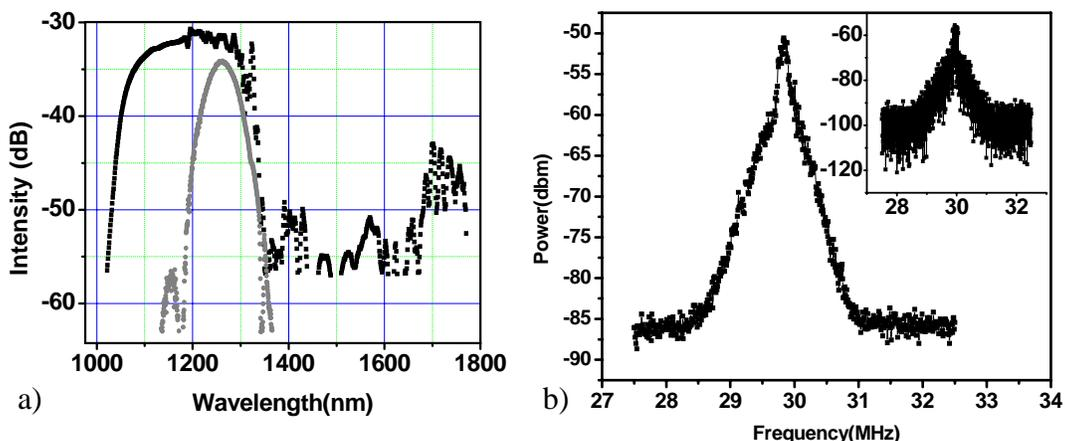
Fig. 2. a) Laser spectrum (grey) and supercontinuum spectrum (black). The spectrum does not show the significant optical power beyond 1.7  $\mu\text{m}$ , where the OSA is no longer sensitive. b)  $f_0$  beat measured on rf spectrum analyzer with RBW of 30 kHz and a reduced video BW. Inset shows same signal, with Resolution BW = Video BW = 30 kHz. (inset). The narrow feature has a width of  $\sim 200$  kHz, and the larger feature has a width of  $\sim 1.5$  MHz.
