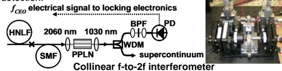
Phase stabilization of the fiber comb is more straightforward than for solid-state systems since the laser pump current can be directly modulated and the cavity length is easily controlled.
