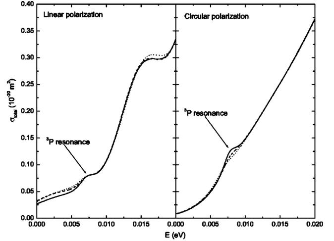
FIG. 1. Total cross section for photodetachment of Cs anions in a static external electric field  $F=20$  kV/cm as a function of the detached electron's energy. Full lines denote exact calculations within the Kirchhoff-integral approach, dotted lines correspond to frame-transformation calculations, and dashed lines stand for the calculation which takes the rescattering effect into account.
