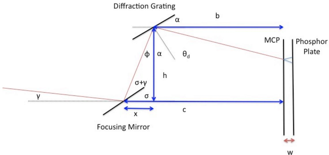
Figure 1: The spectrometer consists of a focusing mirror, diffraction grating, MCP, and phosphor plate. All important angles and distances are indicated on the diagram.
