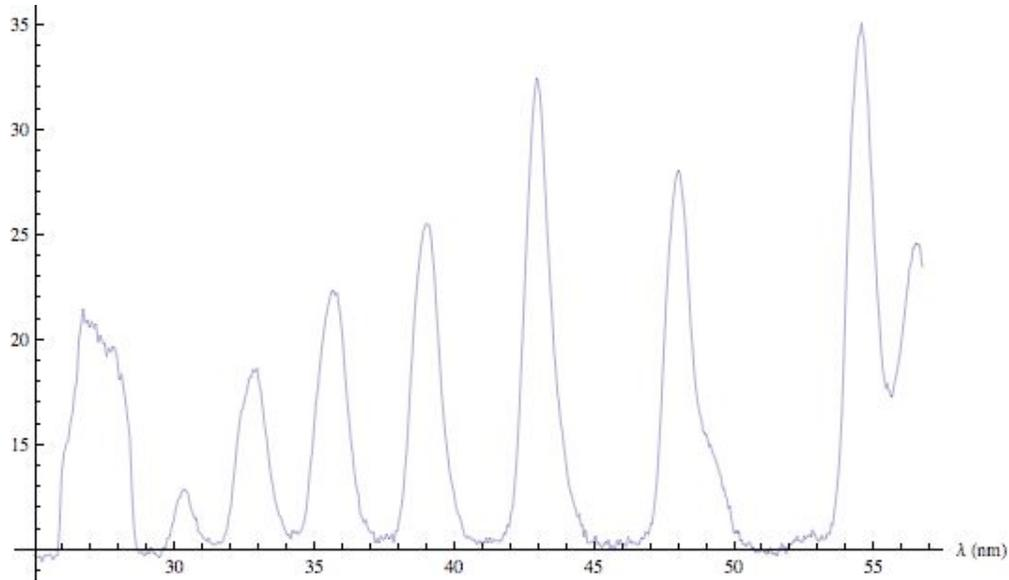
Figure 3 A spectrum generated by High Harmonics Generation. Note the peak smaller than 29 nm is due to a burn mark on the camera that can be seen in the center of Fig 2, this peak does not describe a photon.
