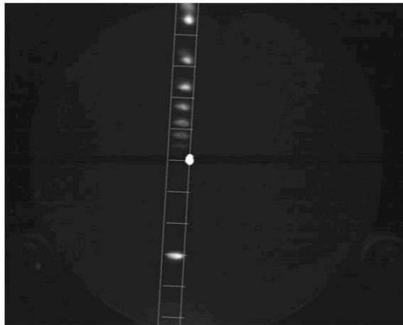
Figure 2: Photograph of spectrum with area of integration outlined. All pixel values between the two vertical lines were summed up in lines similar to the ones shown horizontally.
