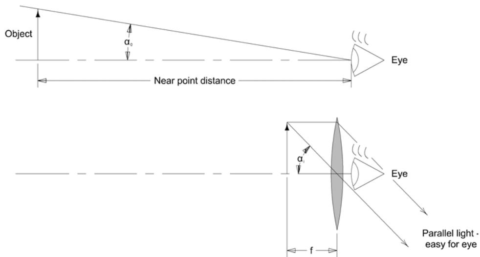
$$\text{Apparent Magnification} \cong \frac{\alpha_i}{\alpha_o} = \frac{\text{near dist.}}{f}$$
