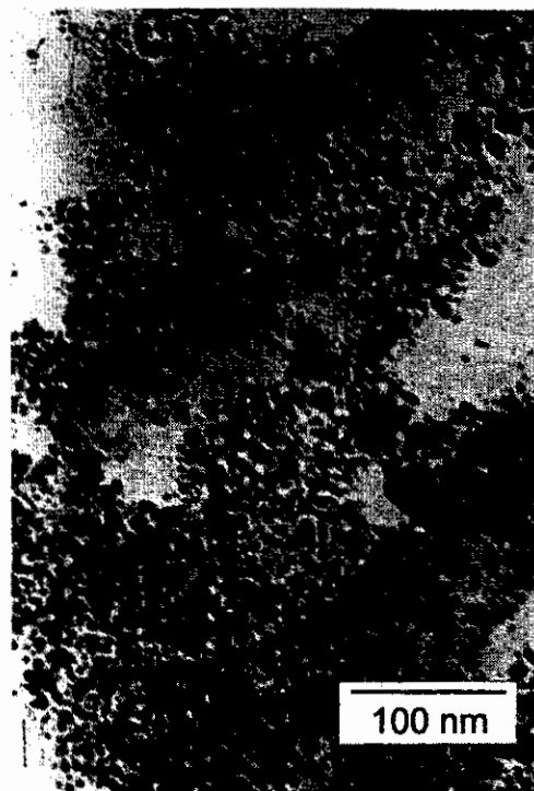
Figure 2. TEM micrograph of gold particles from Au-acetone-toluene-thiol colloid (colloid 1).
