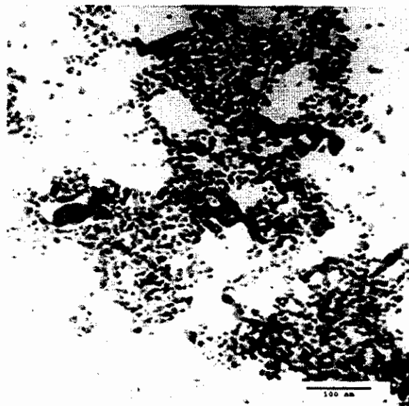
Fig. 11 TEM micrograph of gold-acetone colloid prepared by the SMAD method.
