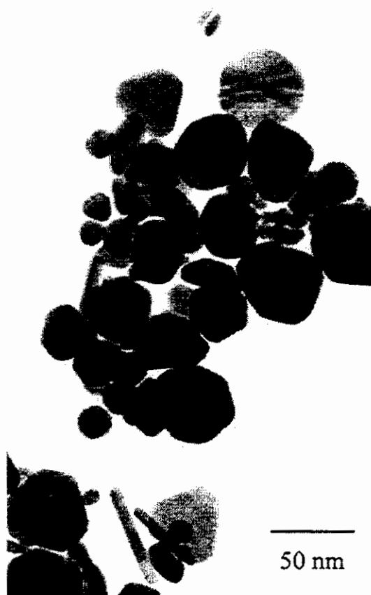
Fig.2 TEM micrograph of an as-prepared gold colloid by the inverse micelle method.
