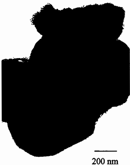
Fig. 9 TEM micrograph of a digestively ripened gold colloid in the presence of octanethiol ( C_8SH ) prepared by the inverse micelle method (sampling is done after the colloid is cooled down to room temperature).
