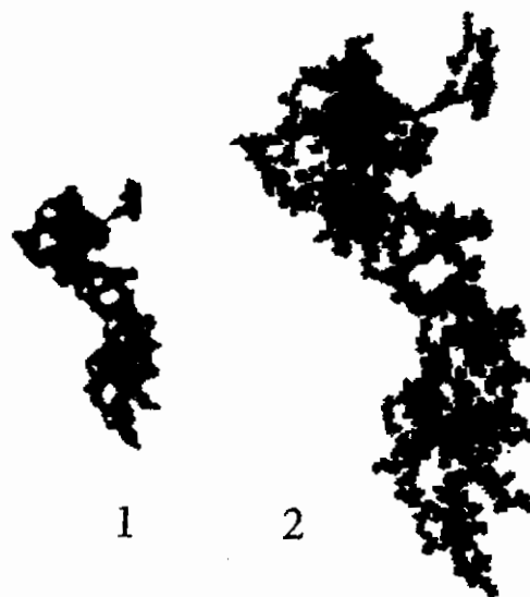
FIGURE 2. Computer-digitized image of a computer-generated DLCA cluster ( D=1.75 ) at two magnifications differing by a factor of two. At magnification two, additional structures are resolved.
