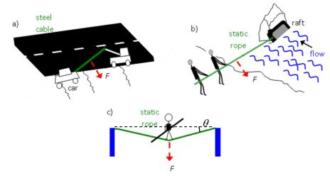
In a) and b) it is advantageous to apply a force to increase the tension in the rope. In c) a sideways force is already present and so the bend in the rope is shown.
