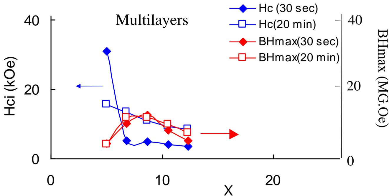
High field magnetization ( $M_s$ ), coercivity ( $H_{ci}$ ) and energy product ( $BH_{max}$ ) as a function of anneal temperature and anneal time for several compositions of initially multilayered  $SmCo_x$ .
