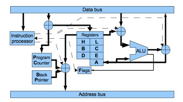
• Counters, "registers", an "arithmetic logic unit", an instruction decoder, and a lot of switches.
