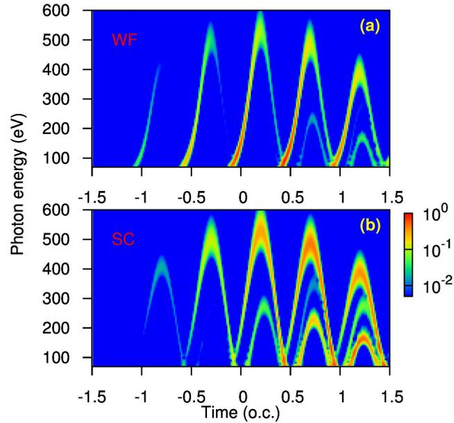
**Supplementary Figure S4: Time-frequency analysis of harmonics in Supplementary Fig. S3(b).** (a) Waveform (WF) and (b) single-color (SC) wave. These figures show the relative strength of harmonic emission from “short”- and “long”-trajectory electrons. (o.c. stands for optical cycle of the fundamental laser, i.e., 4.74 fs for WF and 4.92 fs for SC.)
