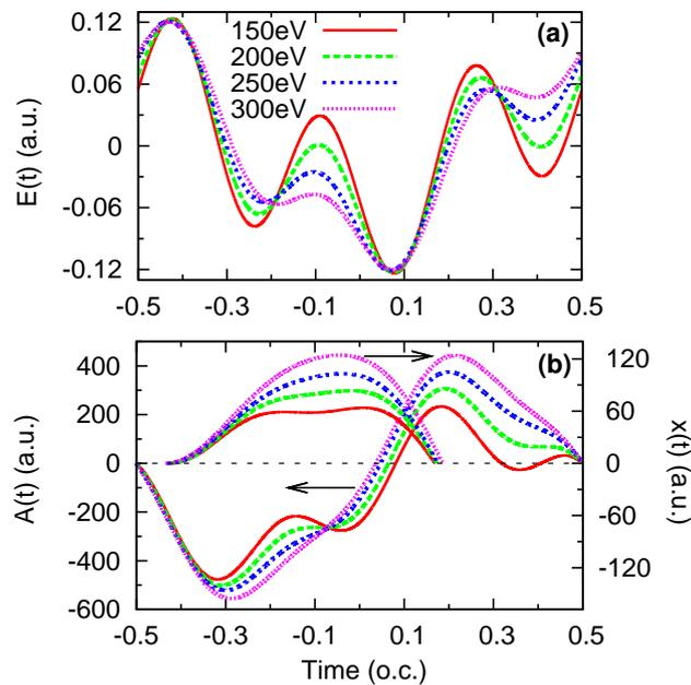
**Supplementary Figure S5: Analysis of the the classical motion of an electron in two-color field that results in different cutoff energies.** (a) The waveforms shown in Fig. 4(b) of the main text. Laser parameters are from Table 4. (b) The corresponding vector potential  $A(t)$  and displacement  $x(t)$  of the electron for electrons that return with the maximum energies. (o.c. stands for optical cycle of the 1600-nm laser.)
