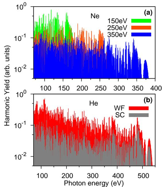
**Supplementary Figure S3: Single-atom harmonic spectra of two-color waveforms.** (a) Single-atom HHG spectra of Ne by using optimized waveforms to generate three different cutoff energies. The corresponding maximum returning electron energies are 150, 250 and 350 eV, respectively. Laser parameters are from Table 2. (b) Comparison of single-atom HHG spectra of He by using waveform (WF) and single-color (SC) wave. The maximum returning electron energy is 500 eV. Laser parameters are from Table 3.
