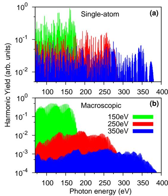
**Supplementary Figure S2: Harmonic spectra of optimized single-color fields.** (a) Single-atom and (b) macroscopic HHG spectra of Ne generated for three different cutoff energies. The corresponding maximum returning electron energies are 150, 250 and 350 eV, respectively. Laser parameters are from Table 2.
