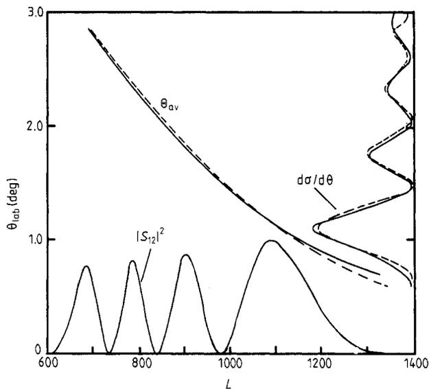
**Figure 4.** Mapping of electron capture probability to obtain differential cross sections via a deflection function. The full curves in the deflection function and in the differential cross sections are obtained from quantal calculations while the same quantities calculated by the semiclassical method are shown as broken curves.
