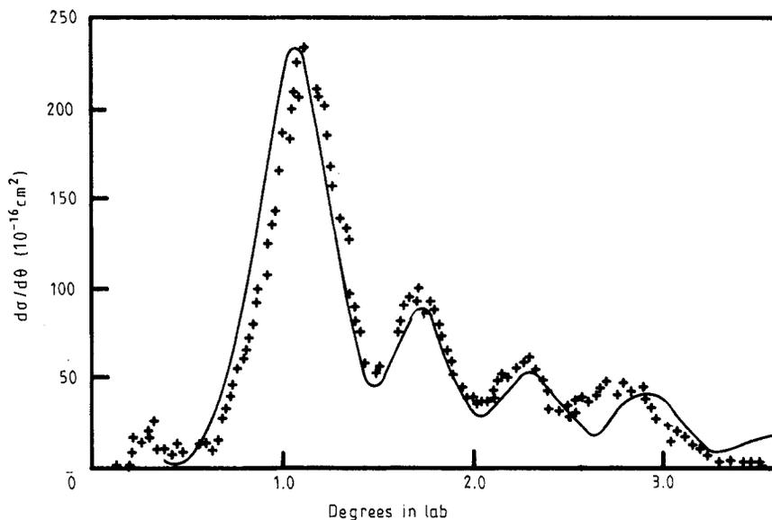
**Figure 1.** Differential charge transfer cross section for  $C^{4+}$  collision on He at 1520 eV (the relative velocity  $V = 0.071$  au). Experimental data are from Tunnell and Cocke (Barany *et al* 1986). The theoretical cross sections are given in units of  $10^{-16} \text{ cm}^2$  and convoluted with experimental resolution (full line). Experimental data are in arbitrary units.
