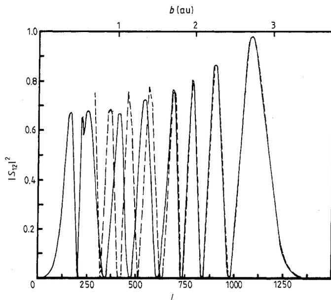
**Figure 3.**  $|S_{12}^l|^2$  against partial waves at impact energy 1520 eV. The full curve is the result of a full quantal calculation. The broken curve is from a semiclassical calculation using a curve trajectory (see text).
