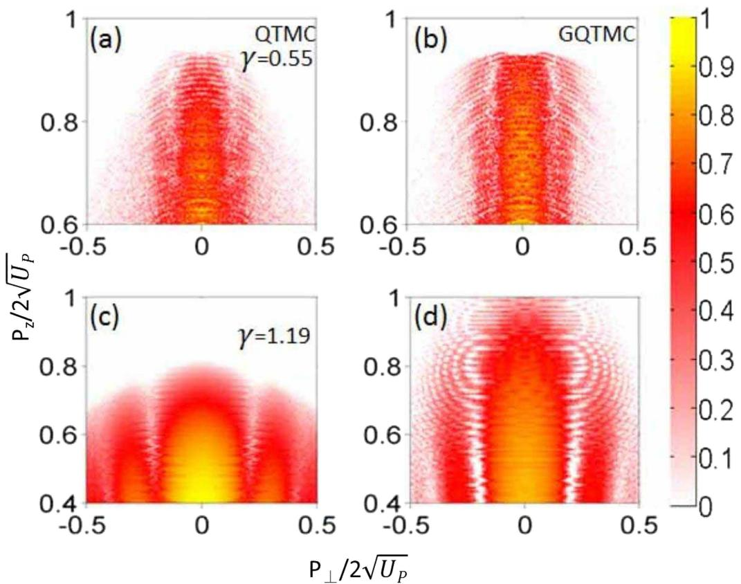
**Figure 4.** Comparison of the final PMD due to ionization from area A (see Fig. 3d) calculated by the QTMC and GQTMC for  $\gamma=0.55$  and  $1.19$ , respectively. The parameters are the same as in Fig. 2.
