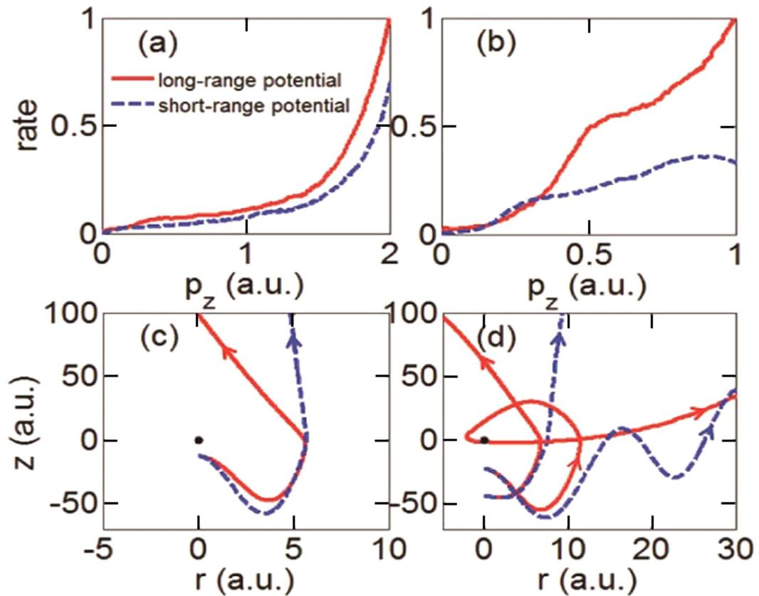
**Figure 6.** Effect of Coulomb potential vs short-range potential on the final longitudinal momentum distribution of the rescattering electrons for  $\gamma=0.55$  (left column) and 1.33 (right column), respectively. Typical electron trajectories are shown for these two regimes also. Note that  $z$  is the longitudinal direction and  $r$  is the transverse direction. The parameters are the same as in Fig. 5.
