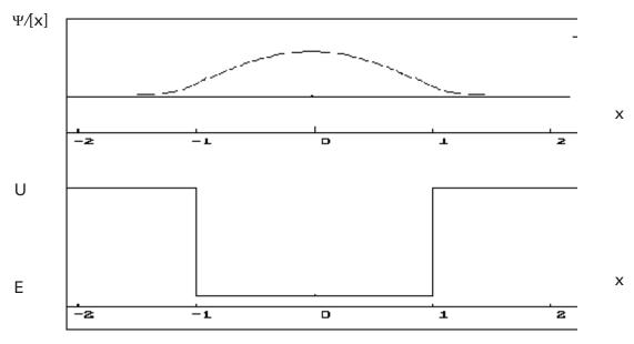
*Figure 4: Diagram of a potential well and its corresponding wave function.*
