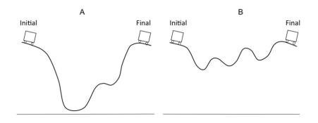
Assume frictional effects can be ignored. How does the final speed of roller coaster cart A compare to the final speed of roller coaster cart B, if the mass of the carts is the same and they both start at rest?
