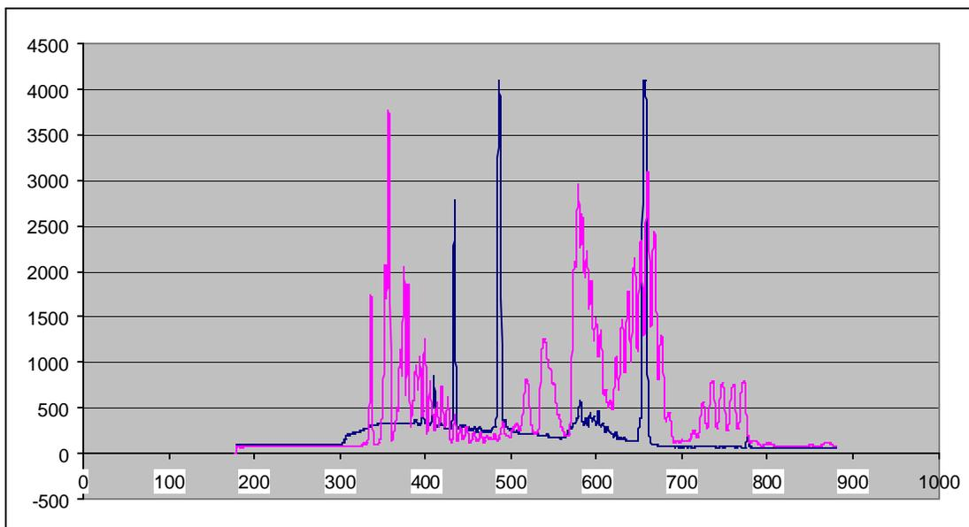
**Figure 18: The hydrogen and nitrogen gas tubes test results. The horizontal axis represents wavelength and the vertical axis represents intensity.**
