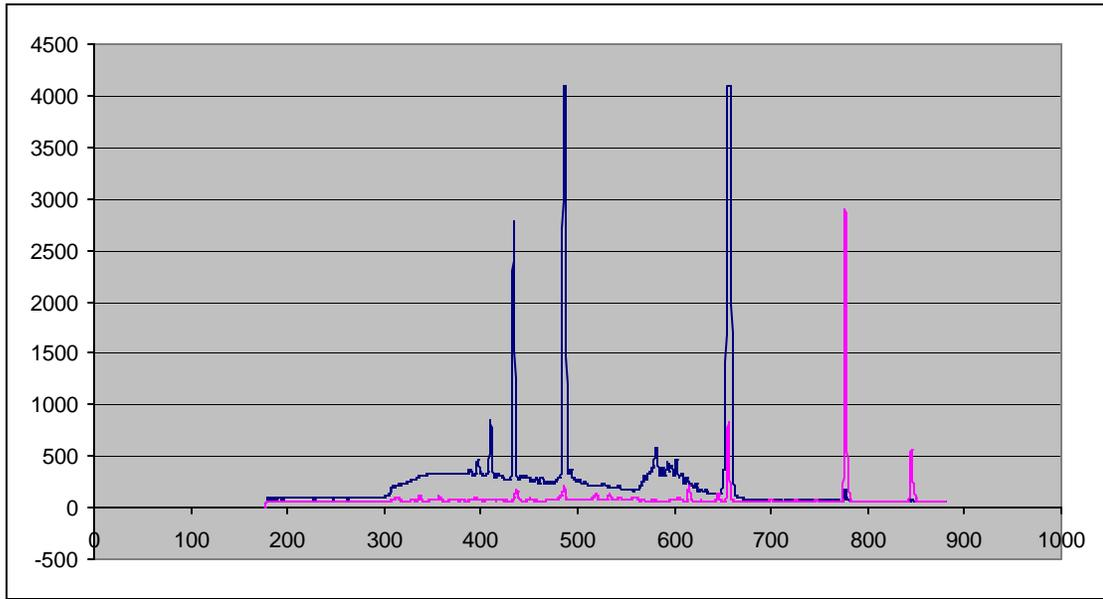
**Figure 19: The hydrogen and oxygen gas tubes test results. The horizontal axis represents wavelength and the vertical axis represents intensity.**
