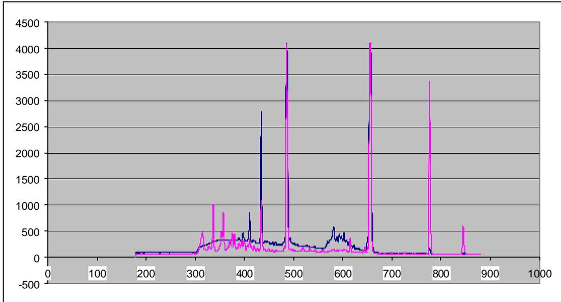
**Figure 21: The hydrogen and water vapor gas tubes test results. The horizontal axis represents wavelength and the vertical axis represents intensity.**
