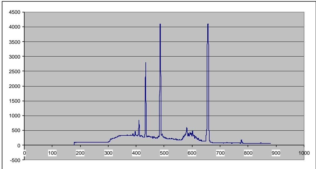
**Figure 17: The hydrogen gas tube test results. The horizontal axis represents wavelength and the vertical axis represents intensity.**
