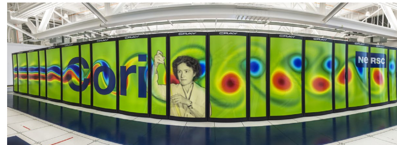
Cori “Haswell” supercomputer with peak performance of 30 petaflops (Floating Point Operations per Second)
