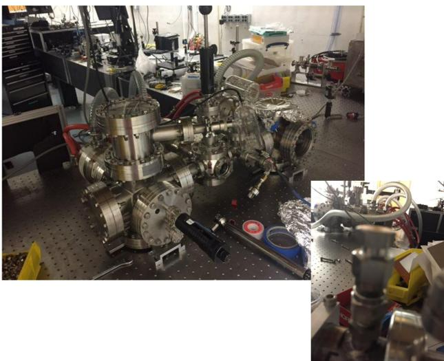
The high harmonic chamber consists of two pumping differential chambers that are connected to two turbo pumps. These turbo pumps allow the pressure to stay constant at  $10^{-6}$  torr. This pressure is needed to keep ambient air out of the chamber and only allow argon gas, the non-linear medium, to be ionized. The pressure is also needed to be low so that the MCP does not become defective and break when exposed to the water vapor present in ambient air.
