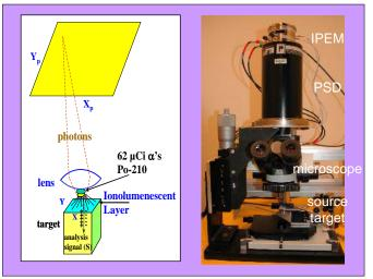
does not have to be focused, which ameliorates the use of costly and complicated nuclear microprobe forming systems. Expensive accelerators can even be avoided by using radioactive sources. Also, because this full-field microscope utilizes light produced by the ions, IPEM can be performed in air or vacuum.
