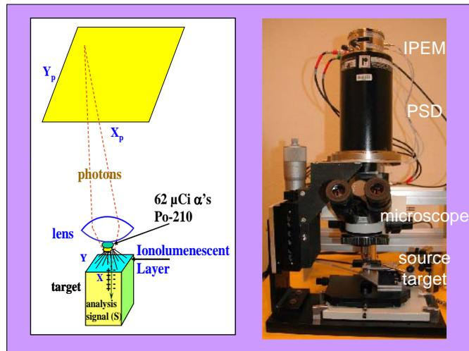
Instead of focusing high-energy ions, the IPEM technique is based on determining the position an individual ion enters the surface of the sample by projection optical microscopy. These position signals are then correlated with the ion-induced signal generated in the sample target or device under test (DUT), such as a malfunction in an integrated circuit or the measurement of charge collection or current transients.
