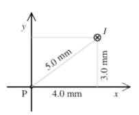
12. (12) A 12.0 cm  $\times$  12.0 cm square coil has 250 turns and carries a current of 4.00 A. A uniform magnetic field of strength 230 mT exists in the plane of the coil as shown.
