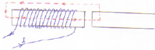
Assume that the fields  $\vec{B}_{\text{iron}}$  and  $\vec{H}_{\text{iron}}$  within the iron are nearly uniform, and that  $d \ll a \ll l$ . The arrangement is surrounded by vacuum. A constant current  $I = 5.0$  A is flowing in the coil.
