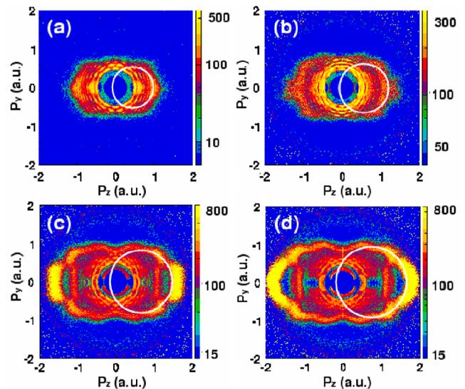
FIG. 2 (color online). Density plots of electron momentum spectra at different laser intensities for 7 fs pulses on Xe. The intensities (in units of  $10^{13}$  W/cm<sup>2</sup>) and corresponding values of  $p_0$  (in a.u.) are, respectively, (a) 4.18, 0.74; (b) 5.8, 0.86; (c) 7.1, 0.95; (d) 8.3, 1.03. The white circles show the inner edges of the regions from which the differential cross sections were extracted (see text).
