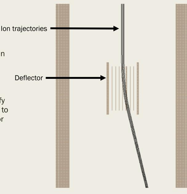
Example of an ion trajectory in Simion
