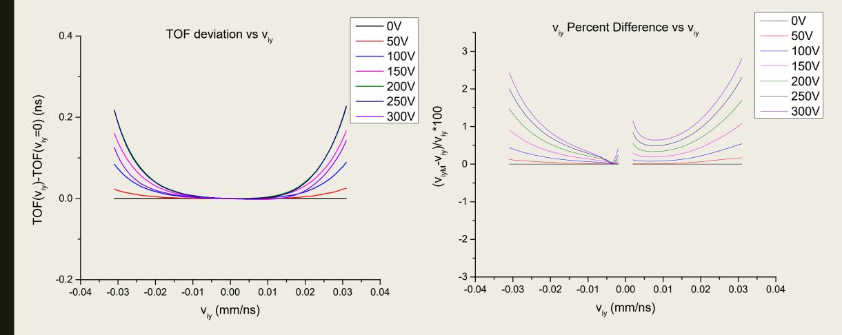
For  $v_{iy}$  less than 5 eV, TOF deviation is less than 0.2 ns. The time resolution of our setup is 0.2 ns. Percent error in velocity is around 2%.
