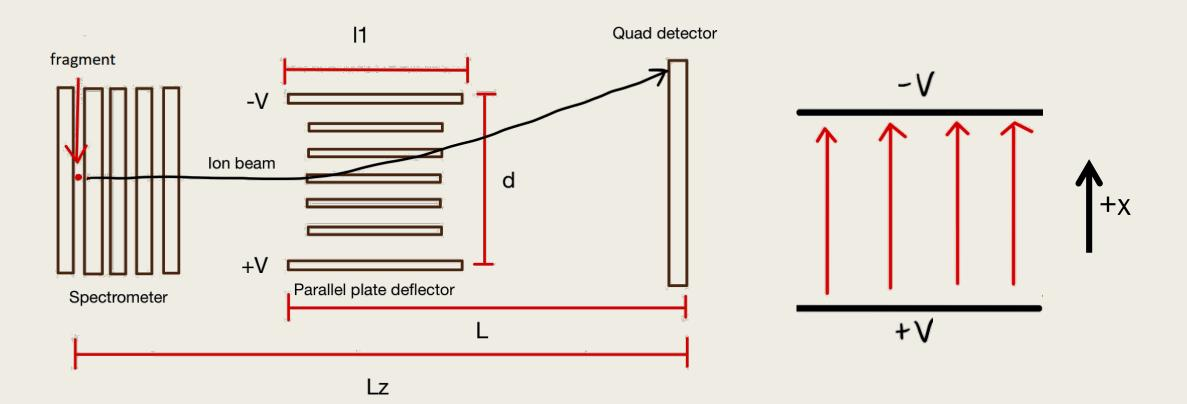
**q** = charge  $E_z = \frac{1}{2} m v_{0z}^2$  **v**<sub>ix</sub> = dissociation velocity in x-direction **TOF** = Time of flight
